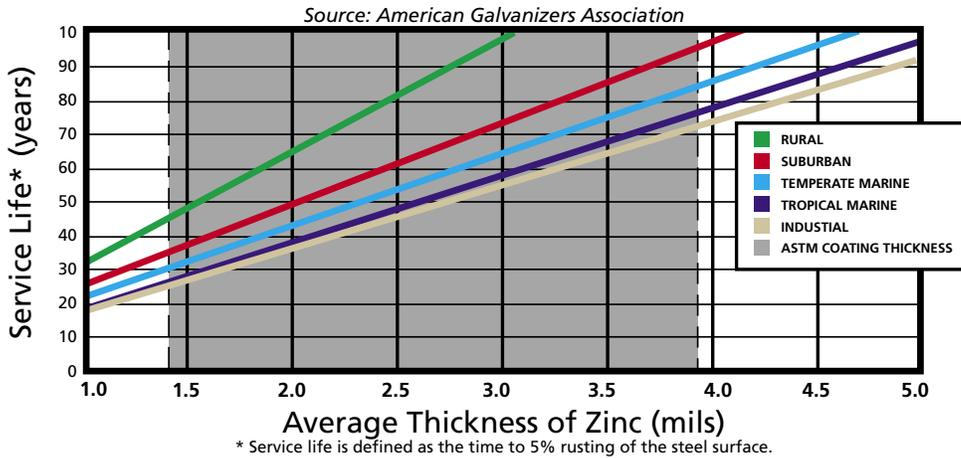
The Service Life Chart (SLC) was developed based on decades of corrosion rate data collected from galvanized steel samples exposed to the five defined environments in cities all over the world, and a corrosion prediction model based on statistical methods and neural network technology.
