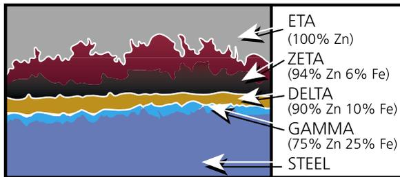
1. After preparation, reinforcing steel is immersed in an 850° bath of molten zinc.
